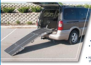
NOTE: Minimum inside door opening required for this ramp is 34". Minimum requirement for floor to ceiling opening 7' ramp - 37", 8' ramp - 41".
