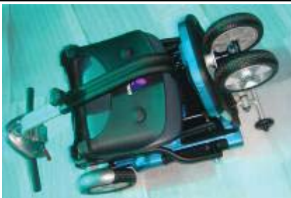
Pull down the tiller to fold the scooter. Push the tiller softly until the tiller locks.
