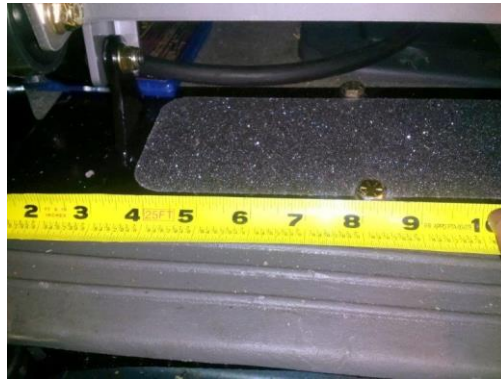
Position bolt 8 1/4" from left side of bracket
