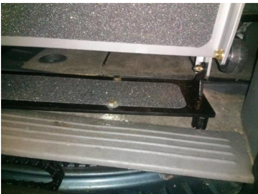
Shimming may be req'd to level ramp (R side)
