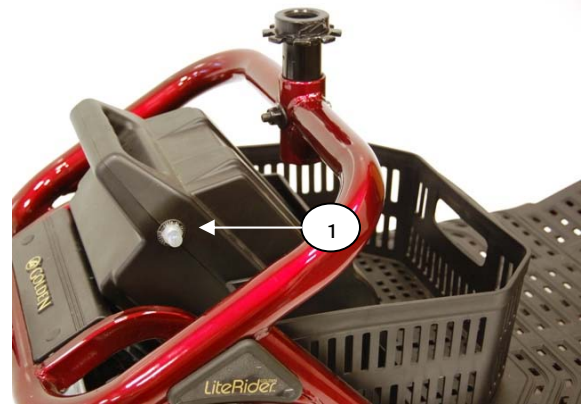
Figure 27. Main Circuit Breaker
