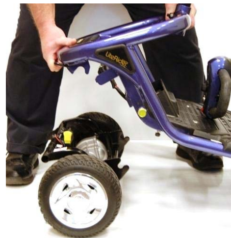
Figure 18. Lifting the Frame
