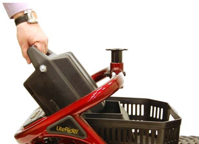
Figure 21. Battery Pack Installation
