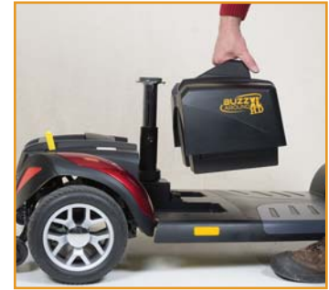
Step 2: Pull out the battery pack!
