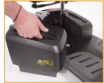
Step 2: Pull out the battery pack!
