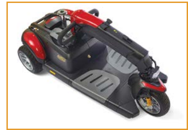
2. The tiller folds easily and locks in place.
